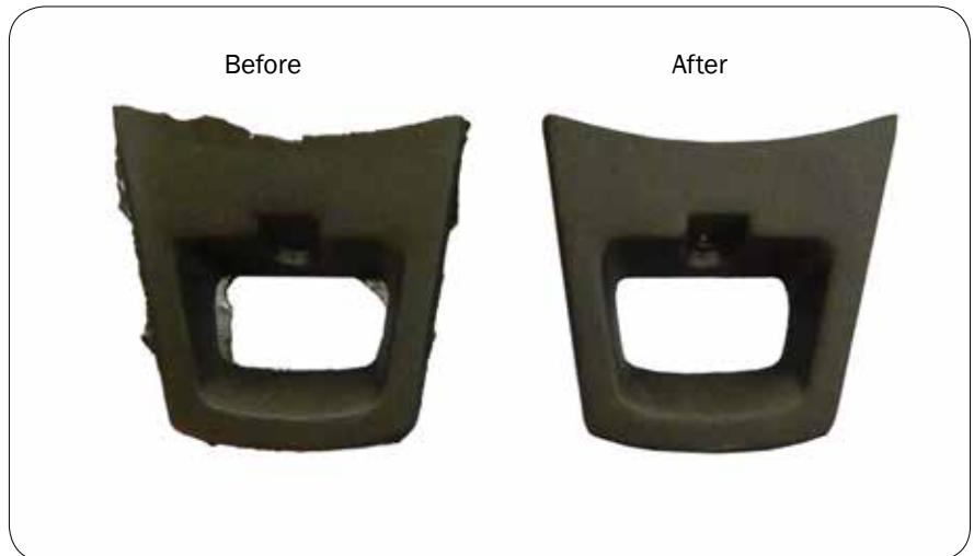
Deflashing of a Bakelite Handle
